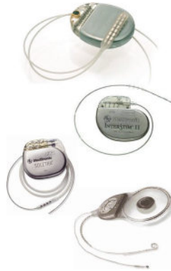
FIGURE 1: Most currently approved and clinically successful neural prostheses use fairly bulky hermetic titanium cans with multiple feedthroughs and polymerically encased flexible leads to relatively large platinum-alloy electrodes, similar to cardiac pacemakers of the 1970s.
